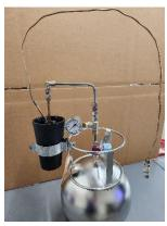
Attach the flow regulator and trap assembly. Regulator standard flow rate is 1 hour. Fill cup with dry ice.
