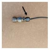
2 micron stainless steel frit is installed at the probe end.
