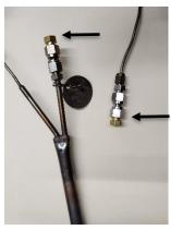
Cap both ends of the trap after sampling.
