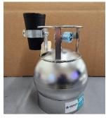
Attach the bracket and cup to the SUMMA canister.
